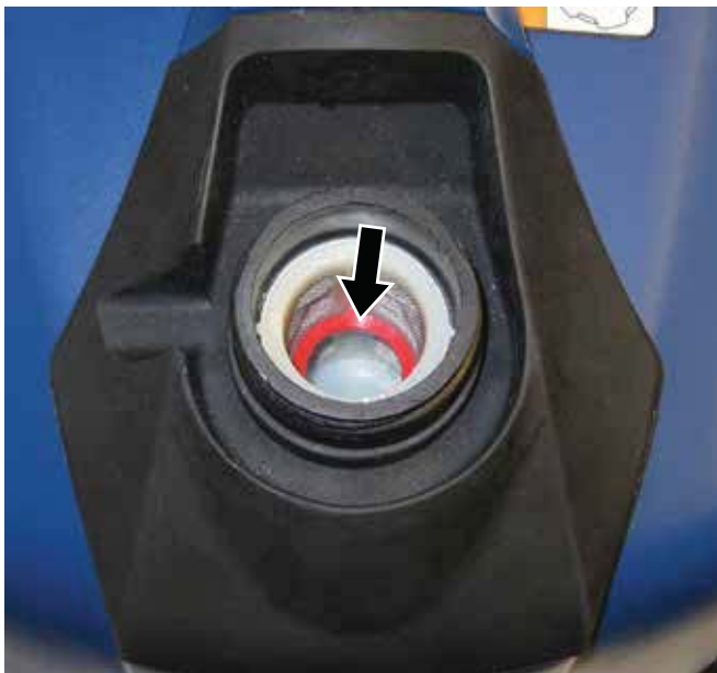
Figure 20 – Maximum Gasoline Fill Level
