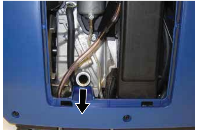
Figure 30 – Draining Engine Oil (WH1000i Shown)
