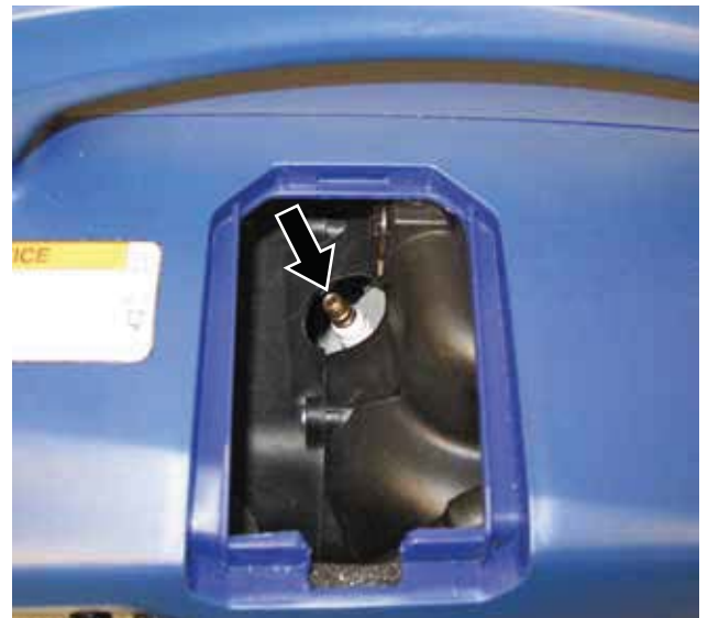
Figure 36 – Removing Spark Plug
